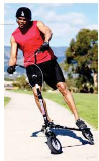
especially the range with which you can rock the steering column left and right. This is especially important because it is exactly this rocking capability that propels the vehicle forward. Get used to letting your arms do the rocking --- not your body.
