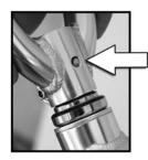
Depress the locking pin and slide the fork the final inch or so until the locking pin snaps into the hole (arrow left).
