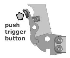
The same procedure also applies to collapsing the vehicle. When Trikke cambering vehicles are new, sometimes the joints are tight. This is normal, and they will loosen up after some use. If tightness continues, use some spray oil like WD-40 to lubricate the joints.
