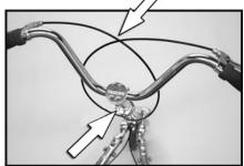
Position the handlebars with the brake cables crossing once behind the steering column and again in front (see white arrows left). This simple method insures that the left brake lever actually operates the left rear brake. If you find that your brakes are crossing, please start again and properly mount the handlebars
