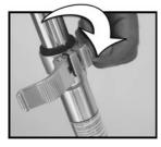
If the quick release is loose, use the adjustment finger nut to tighten the quick release. Properly adjusted, it requires a firm hand to close.
