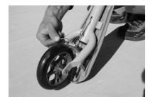
First, loosen the 2 bolts that hold the brake cable to the pad. Pull the cable towards the front (follow arrow) until the pad is close to the tire - leave a gap, so the wheel spins freely - 3 mm (1/8") - The desired result is to keep the brake pad as close to the wheel as possible without rubbing. Keeping your cables tuned like this will optimize the operating effectiveness of your brakes. Tighten the bolts back.
